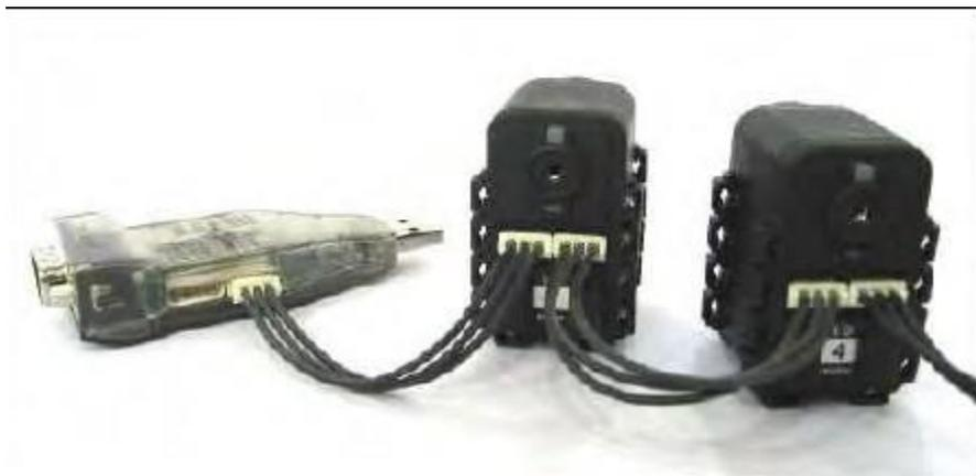
**Photo 4.4.USB to serial convertor and daisy chain connection.**
