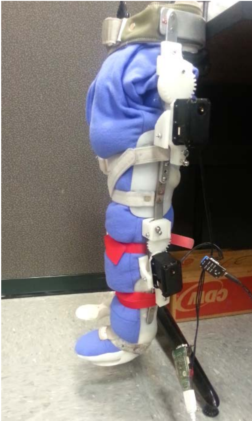
Figure 3 - Full system test was run using footed pajamas filled with 10 lbs of rice to simulate a weighted leg. This was done to confirm the design could perform the necessary motions while subjected to an expected load.
